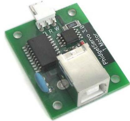
The PhidgetServo boards are our most popular Phidgets; we sell lots of these. They can control most Remote Control (RC) servo motors, with an accuracy of 0.1 degrees, directly from your PC.
