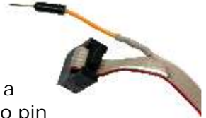
Arduino-as-ISP trick needs a hacked cable
