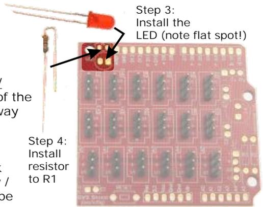
**Step 4 - 470 ohm Resistor (Yellow / Violet / Brown):** Fold over one leg of the resistor so it's pointing the same way as the other lead, and install it to position R1.
