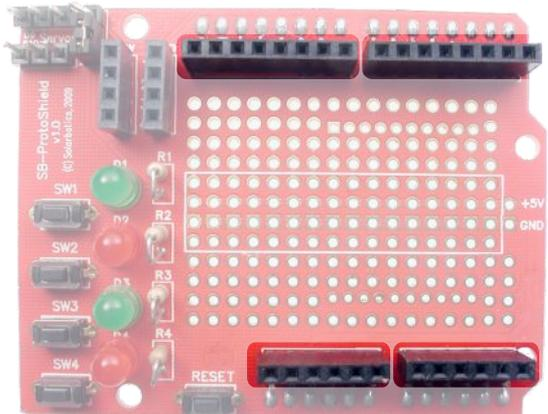
**Step 7 - Install the 6 & 8 Pin Female Header Sockets:** These are only really of interest to you if you'll be using the mini-breadboard (which is most applications). These headers make it really easy to quick-prototype up a new idea. Use the same technique as in Step 6.
