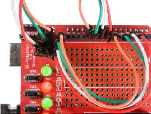
Hook up your protoboard like this, download our sample code (from [http://bit.ly/SB\\_16090\\_Code](http://bit.ly/SB_16090_Code)), and feed it to your Arduino. Press to turn on, press to turn off!
