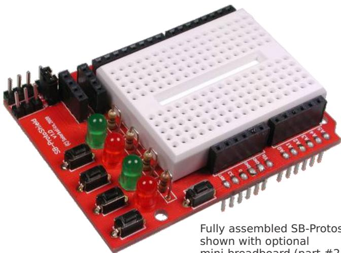
Fully assembled SB-Protoshield shown with optional mini-breadboard (part #21380)
