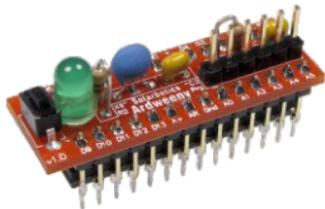
**Ardweeny:** It's a breadboard-friendly, *inexpensive* Arduino-clone. Add your own TTL-compatible programming cable, and get join the Arduino revolution!
