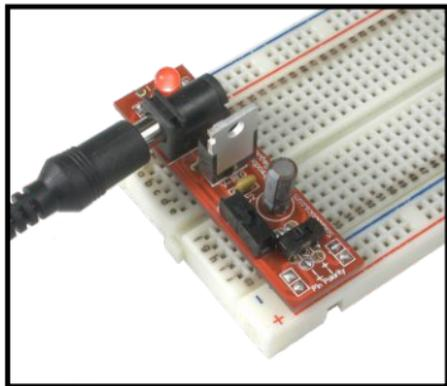
The BVR has been specially designed to mount onto the power rails of a standard breadboard and accepts any standard 2.1 mm barrel plug found on most AC adapters. This makes it ideal for many prototyping projects!
